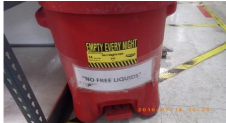
Properly manage recyclable solvent-contaminated wipes
